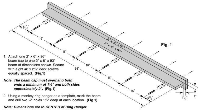
3. Install six monkey ring hangers and six chains with two 1/4" x 11/2" lag screws each. (Fig.1)
